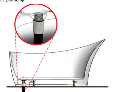
**5.** Apply silicone under the 4 legs of the bath, and the appropriate glue on the connecting joint (PVC). Install the bath in its final position.
