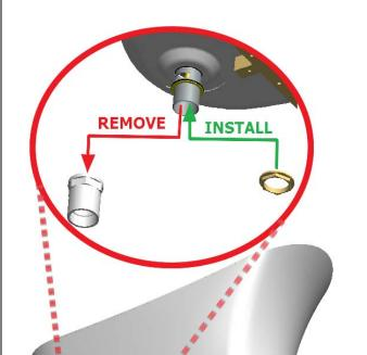
**8.** Install the ITD35 following the installation instructions provided with the floor drain.
