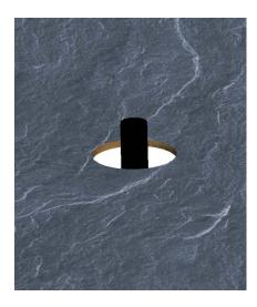
**4.** Make a test without applying glue, to ensure the correct height of the plumbing.
