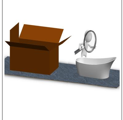
**2.** Place the bathtub in its final position. Adjust the legs so that the bathtub rests on its 4 legs, the skirt not touching the ground.
