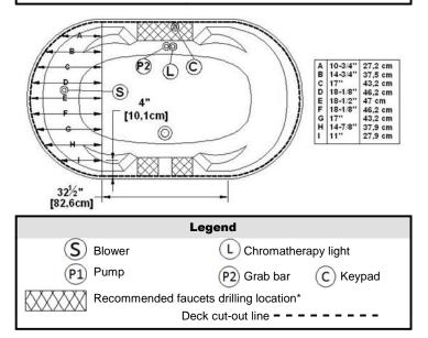
\*It is possible to install the faucets elsewhere on the product. The installer must verify that there are no piping or wires before drilling.
