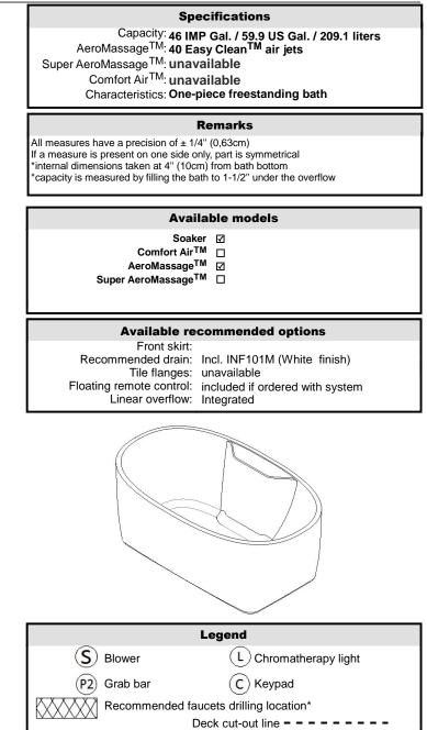
\*It is possible to install the faucets elsewhere on the product. The installer must verify that there are no piping or wires before drilling.
