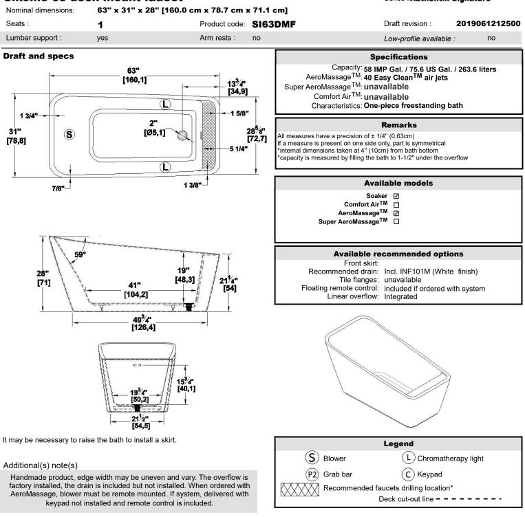
\*It is possible to install the faucets elsewhere on the product. The installer must verify that there are no piping or wires before drilling.
