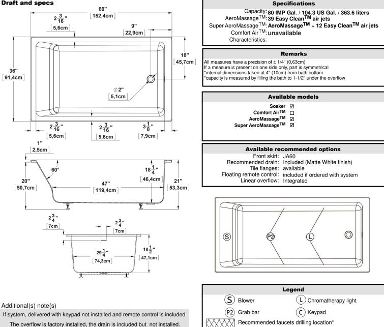
\*It is possible to install the faucets elsewhere on the product. The installer must verify that there are no piping or wires before drilling.
