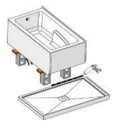
**7.** Make sure there are 2 studs in the following locations (one at the end of the base, the other next to the bathtub's side). These studs will be necessary for the installation of the door wall jambs.
