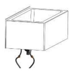
**4.** Place the bathtub on blocks above its final position. Make required connections (hot/cold water, chromatherapy light, keypad, water detector, blower). The blower can be relocated away from its position inside the skirt, to allow an easy access. Test water supply connections and test drain to make sure there is no leakage. After testing, use a small container to collect water under the bath.
