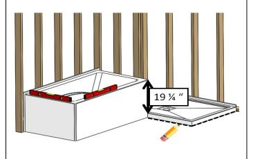
**2.** Remove the bathtub and install the base as described in the Installation Manual provided with the base.
