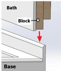
**2.** Remove the bathtub and install the base as described in the Installation Manual provided with the base.
