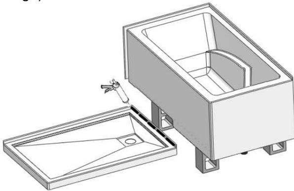
**6.** Remove the blocks and place the bathtub in its final position, and connect the drain.
