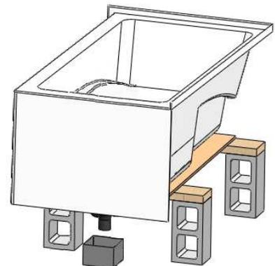
**5.** Apply a generous line of silicone on the side of the base where it comes into contact with the bathtub (along the tiling flange).
