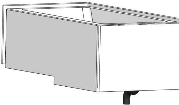
**4.** Place the bathtub on blocks above its final position. Make required connections (hot/cold water, chromotherapy light, keypad, water detector, blower). The blower can be relocated away from its position inside the skirt, to allow an easy access. Test water supply connections and test drain to make sure there is no leakage. After testing, use a small container to collect water under the bath.
