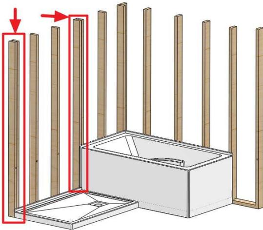
**8.** Secure the bathtub in place by fastening drywall screws into the studs above the bathtub flange
