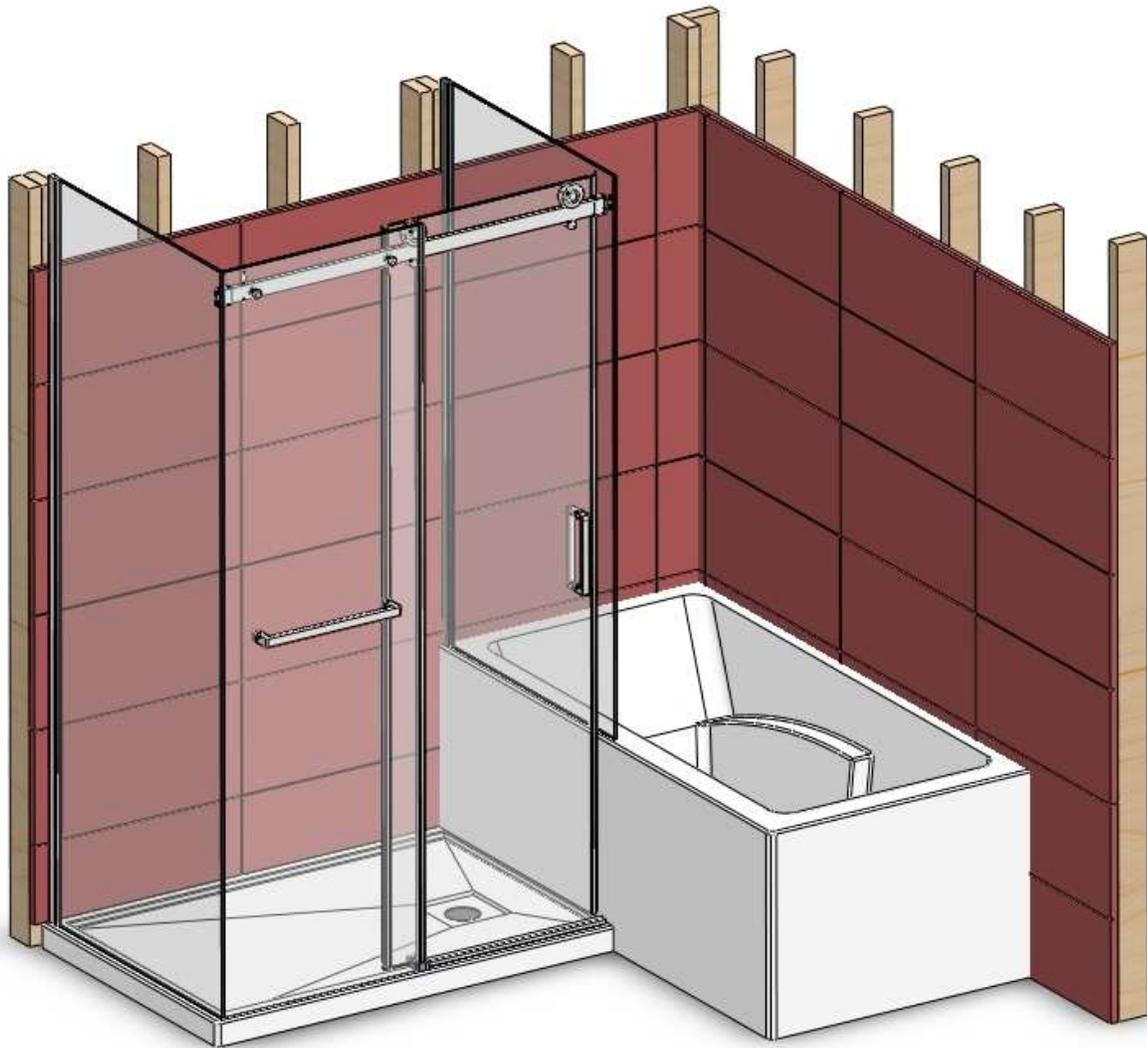
**1.** Place the bathtub and the base in their final position. Adjust the legs of the bathtub so that they support the tub. Make sure that the tiling flange of the base is well inserted immediately behind the block.
