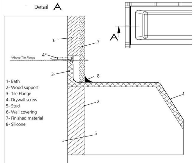
9. Proceed with the installation of the drywall and the ceramic.
