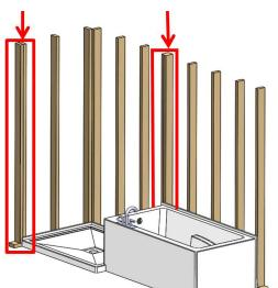
**8.** Secure the bathtub in place by fastening drywall screws into the studs <u>above</u> the bathtub flange.
