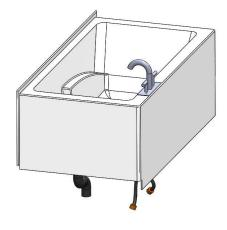
**4.** Place the bathtub on blocks above its final position. Make required connections (hot/cold water, chromatherapy light, keypad, water detector, blower). The blower can be relocated away from its position inside the skirt, to allow an easy access.
