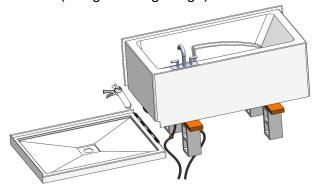
**6.** Remove the blocks and place the bathtub in its final position, and connect the drain.
