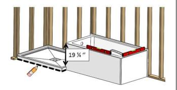
**2.** Remove the bathtub and install the base as described in the Installation Manual provided with the base.
