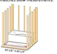
**3.** Place the bathtub and the base in their position. Leave a 1/8" space (3 mm) between the skirt and the tub. Mark the position of the base.
