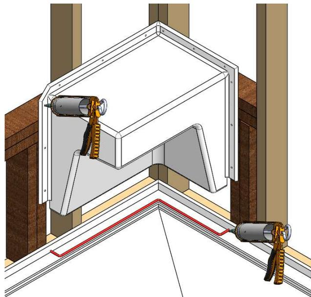
**5.** Position and secure the seat using screws #8 by 1 1/2" in length. Do not tighten the screws too much, it could break the tile flanges.
