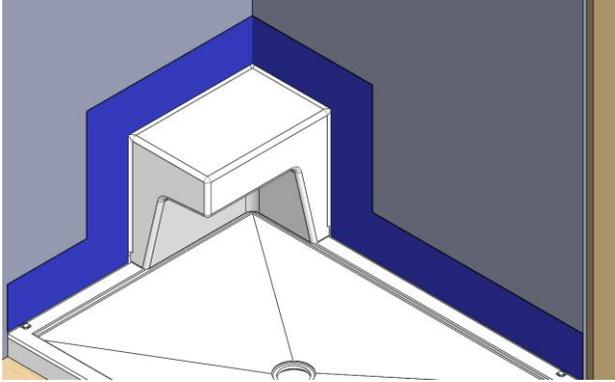
8. Finish the wall (tiles). Make sure to place the tiles on the seal guard (small bump of 1/8" high).
