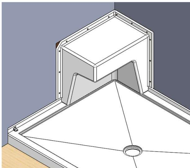
7. Install a waterproof membrane (not provided by Oceania) on drywall and tile flange. The membrane should make contact with about 5" (127mm) of the drywall and 1" (25.4mm) of the tile flange. It is the installer's responsibility to seal the junction between the drywall and the tile flange.
