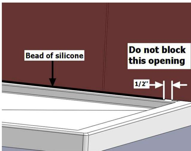
10. Fill the outer portion of the opening with silicone (between the outside of the base and the guard). Make sure that the silicone goes all the way behind the ceramic. Let it dry or cover the silicone and proceed with shower doors installation.
