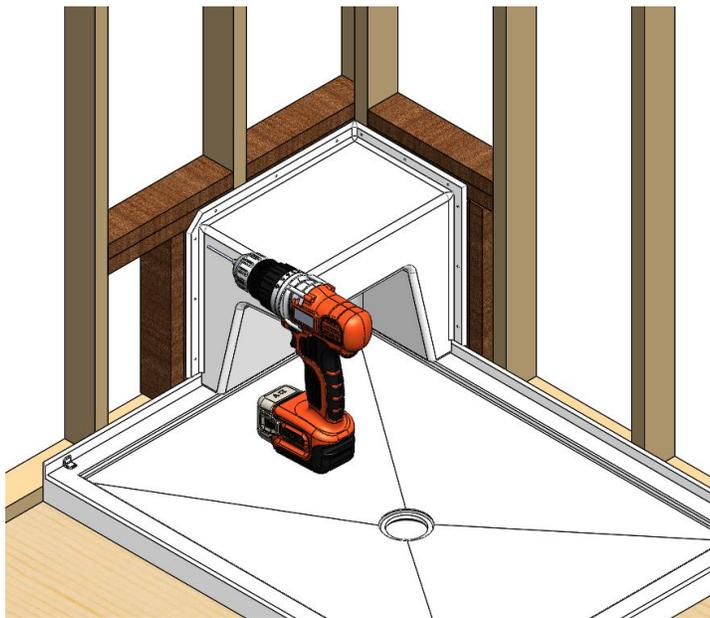
**4.** Remove the seat, apply a bead of silicone on the shower base and in each of the holes in the tile flange.
