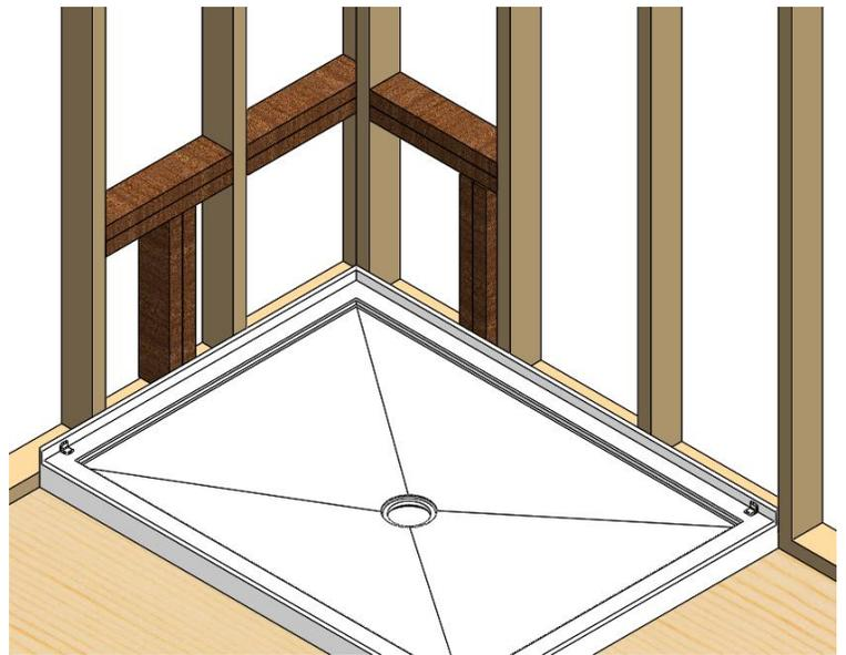
**3.** Place the seat in position, well supported on the shower base and the studs. Using a 1/8" drill bit, drill in the tile flanges next to the studs. Do not drill into the studs (2x4).
