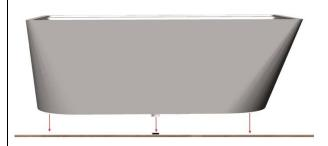
**6.** Apply a silicone suitable for a humid environment (anti-mold) at the junction of the walls and the bath to seal it.
