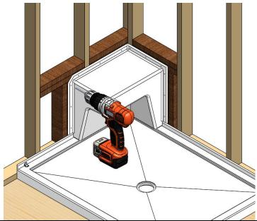
**5.** Position and secure the seat using screws #8 by 1 1/2" in length. Do not tighten the screws too much, it could break the tile flanges.
