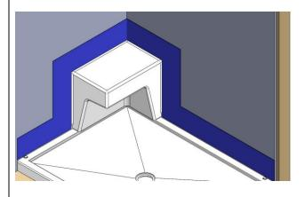
**8.** Finish the wall (tiles). Make sure to place the tiles on the seal guard (small bump of 1/8" high).
