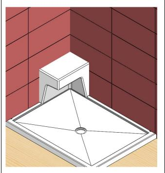
**9.** Once the ceramic is installed, apply a bead of silicone between the base and the ceramic but leave a minimum opening of 1/2" (12.7 mm) between the inside of the base and seal guard.
