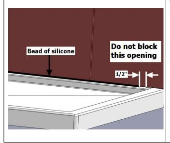
**10.** Fill the outer portion of the opening with silicone (between the outside of the base and the guard). Make sure that the silicone goes all the way behind the ceramic. Let it dry or cover the silicone and proceed with shower doors installation.
