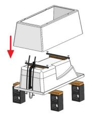
5. Flip the bath/skirt assembly on the blocks. Make required connections (hot/cold water, chromatherapy light, keypad, water detector, blower). For certain models, the blower should be installed somewhere else than under the skirt to allow an easy access to it.
