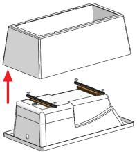
3. Install faucet, drain and overflow. Use flexible hoses for hot and cold water supply. Make sure the overflow is narrow enough to fit between the bath and the skirt.
