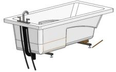
4. Flip the bath upside down on blocks and re-install the skirt with the screws removed in step 2.
